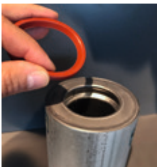
1) Remove sealing ring before welding
