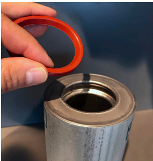
1) Remove sealing ring before welding
