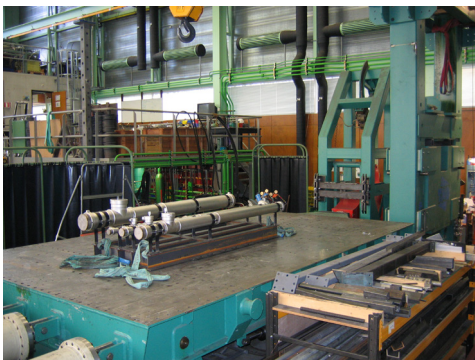
Test set up for the shock test
