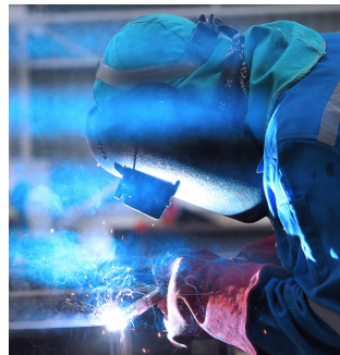
2) Weld the penetration/ drain to the deck/bulkhead
