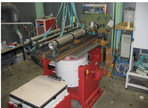
Test set up for the vibration test
